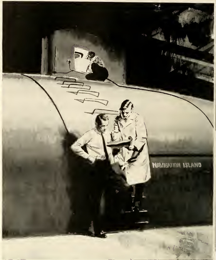
FULL-SCALE SUB SIMULATOR duplicates complex navigational equipment that will guide actual Polaris submarines. To fit systems in restricted space, everything from cabling to 62-ton Gyroscopic Stabilizer must be "engineered" into the bull.
